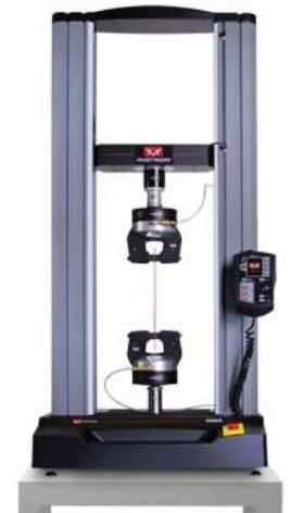
Instron 5966 Mechanical properties
