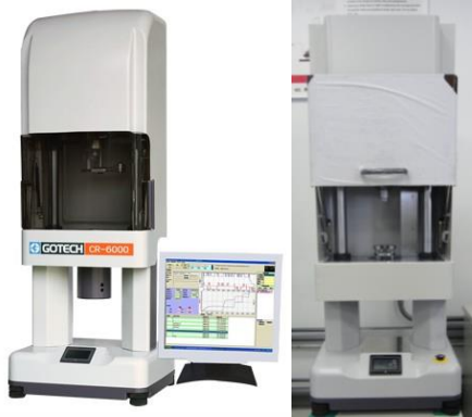
CR-6000 Capillary viscosity at different temperature and shear rates pvT-6000 pvT change at different temperature and pressure
